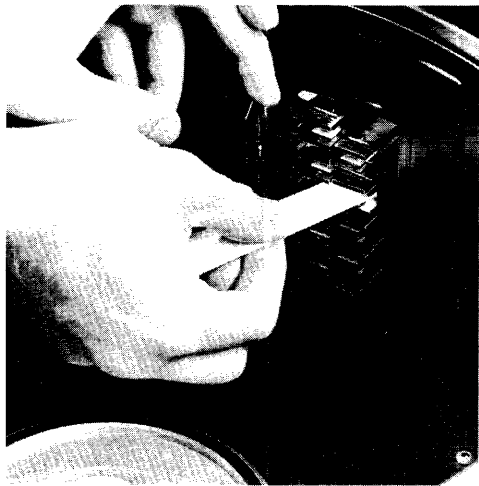
FIGURE 4-3. CLEANING HEADS IN DRIVE
