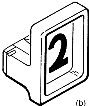
FIGURE 2-12. LOGICAL ADDRESS PLUG
